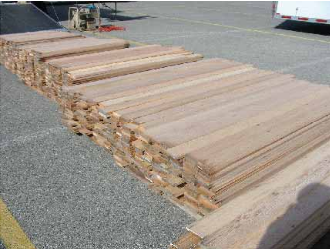
Figure 2.14 Clean, salvaged Douglas Fir, ready for another home.
