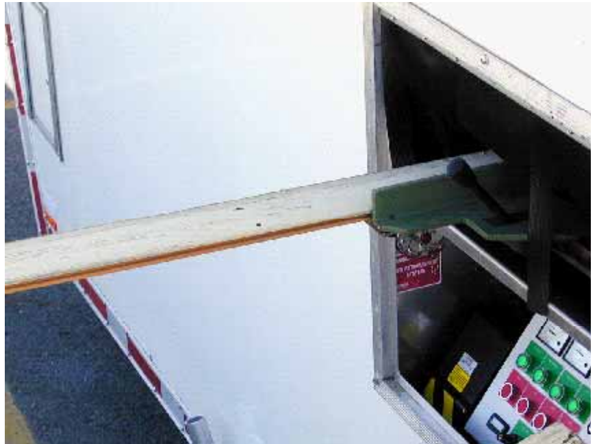
Figure 2.12 Recovered lead painted siding is fed into the planer on one side of the trailer
