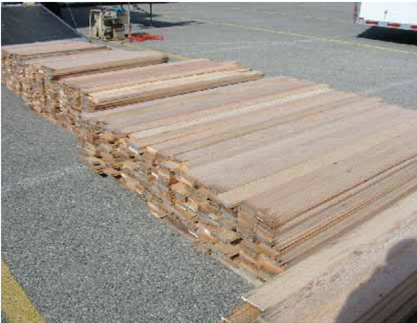
Figure 2.9 Reclaimed old growth lumber, denailed and planed, ready for new construction.
